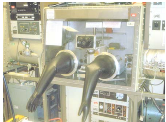
Fig. 1 – Glove box used to work in a controlled environment. Note the microscope above the gloves in this version.
