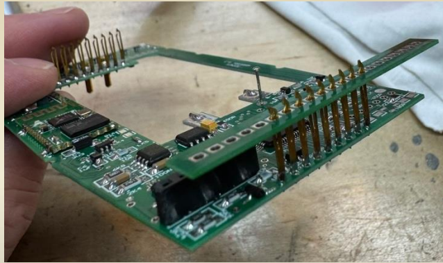
Soldering new pins using alignment tool
